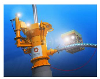
Transportation System and the EC-Drill® Managed Pressure Drilling system.
